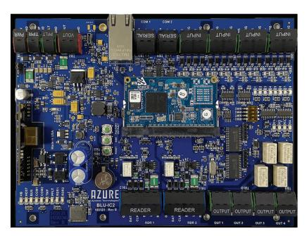
The high performance BLU-IC2 is an open -hardware architechture with embedded Linux TM OS. Communication is encrypted end-to-end (from host down to reader), firmware is encrypted, and user certificates are suported.
