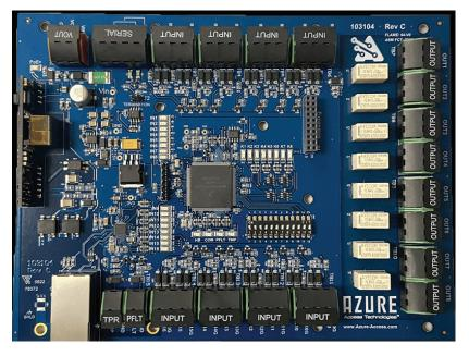
Extend your Access Control system with the Azure BLU-IO 168's 16 high precision sensor inputs and 8 relay outputs. The large number of inputs and outputs enables the full control of additional doors, monitoring extensive sensor networks and elevator control. The BLU-IO168 communicates with OSDP protocols, fully encrypted. Relative to the quantity of hardware interfaces, the BLU-IO168 consumes minimal power.
